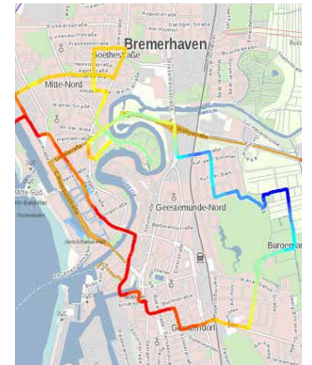
Lufttemperatur 2,0 m in °C 18,1-18,5 18,6-19,0 19,1-19,5 20,1-20,5 20,6-21,0 21,1-21,5 21,6-22,0 22,1-22,5 22,6-23,0 23,1-23,5 23,6-24,0 24,1-24,5 24,6-25,0 25,1-25,5 25,6-26,0 ABB. 40 Profilmessfahrt in Bremerhaven am 25.8.2016 (abends)
