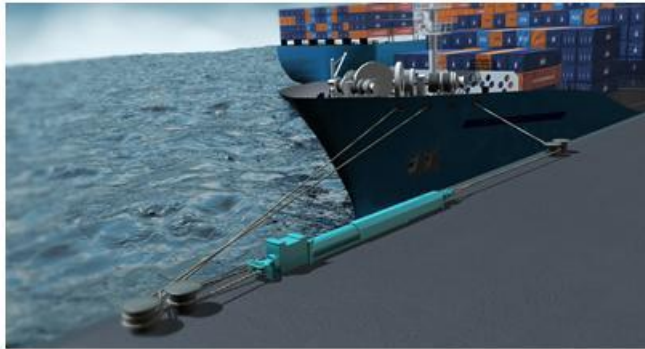
ShoreTension Connected to the FWD breast line
